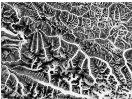
Fig. 6. Multi-scale negative-openness measure for the Shimshal valley in northern Pakistan. This metric highlights the drainage network and valley floors. Other methods can also be used to assess and map the drainage network.
