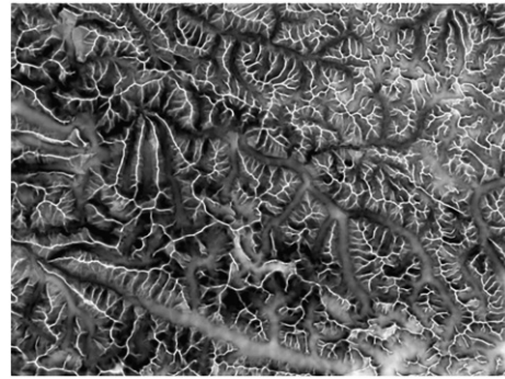
Fig. 5. Multi-scale positive-openness measure for the Shimshal Valley in northern Pakistan. Dark grey tones represent more relief, while lighter grey tones depict less relief (e.g., on ridges). The metric is an average value of the maximum relief angle for eight different directions and accounts for scale variations in relief. It essentially produces meso-scale relief information.
